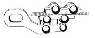
General: For safe and careful installation, tensioning or pulling of ropes. The tension spring construction allows to position the clip on the rope without any additional fixing and maintains the grip on the rope even if the rope is unloaded. Nominal size: 4-10 with round hole Nominal size: 16-38 with oval hole
