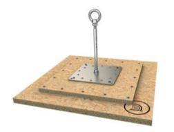
Stainless steel anchor point ABS-Lock X-H-16 (Ø 16 mm) is a fall protection solution for screwing onto OSB or wooden panelling. It is equipped with a base plate (200 x 200 mm) and screwed straight onto the wooden panelling using 16 stainless steel screws. Standard package includes 16 high-quality screws and installation set.
